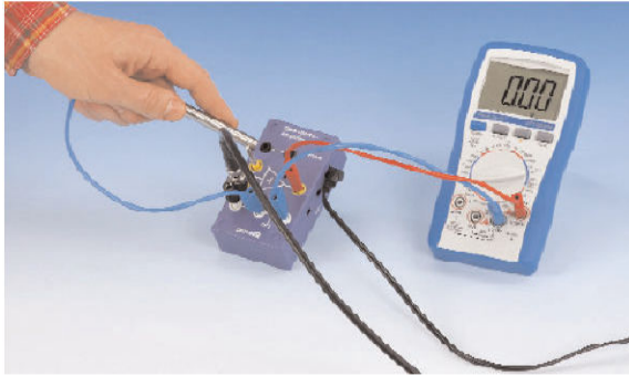
Figure 6: Connection of the electrometer amplifier
